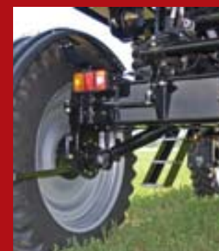
Welded box style leg construction
