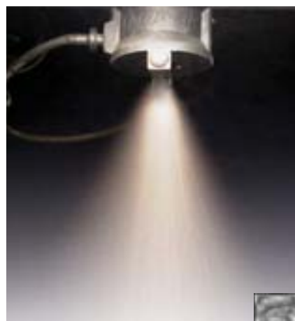
Droplet size set at 100/120 microns.
