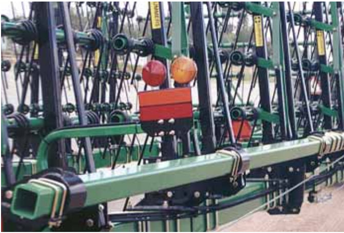
Standard lighting for safe transport on roads.
