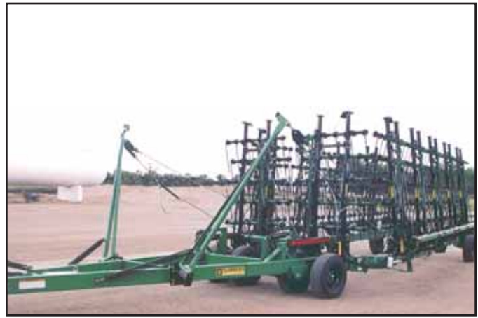
Folded compactly for safe transport.
